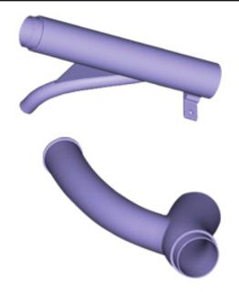
The lab chose the process because it can model with PC (polycarbonate) and PPSF (polyphenylsulfone). These thermoplastics work well for functional testing, which is important for demanding applications, like aerospace.
