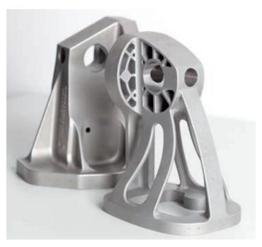
Further example of improved part design: prototype of a topology optimised Airbus A380 bracket made of stainless steel powder produced via DMLS with conventional bracket behind (Source: EADS). waste produced during the atomization process.
