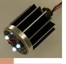
It is well established that keeping the temperature of electronic components below safe temperature limits helps to maintain a long service life and avoids early product failure. The preferred method of achieving this cooling is via the natural convection of buoyancy driven air-flows induced by the electronic heat sources. This method is low cost to implement, simple to maintain and produces zero noise or electro-magnetic interference that can degrade product performance.
