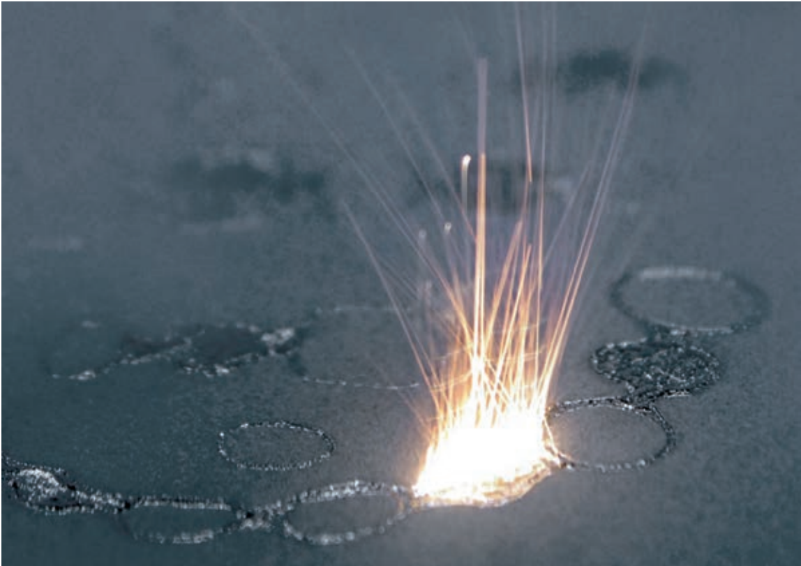
Digital Manufacturing: the laser fuses the metal powder layer by layer at 200 W and a temperature of 1400°C (Courtesy EOS GmbH).
