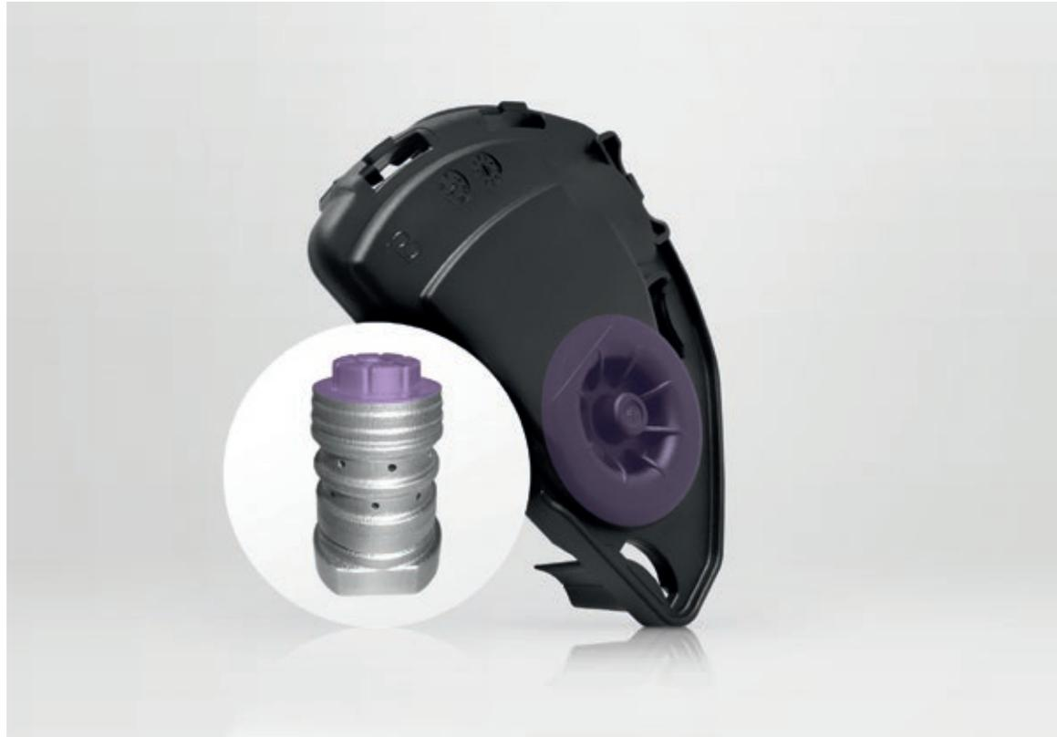
*Tool insert and injection-moulding component: Thanks to conformal cooling the cycle time was reduced and the quality of the housing part improved (Source: LBC, FWB)*
