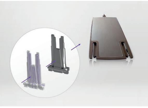
Tool insert and injection moulding component: thanks to conformal cooling the cycle time was reduced by 17% and the quality of the armrest part has been improved (Source: Innomia, Magna).
