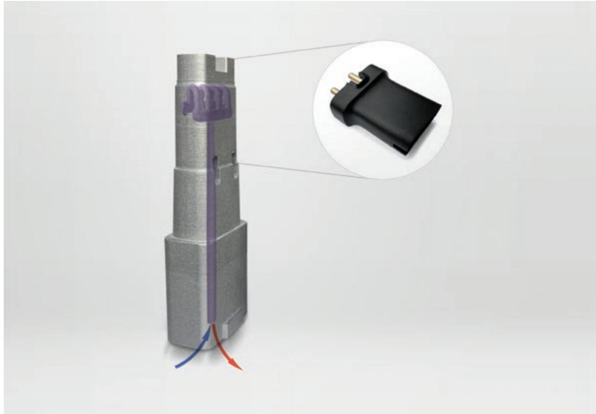
*Tool insert and injection-moulding component: Thanks to conformal cooling the time required for cooling was reduced from 14 to just 8 sec for each production cycle and the quality of the final part improved (Source: Salcomp).*
