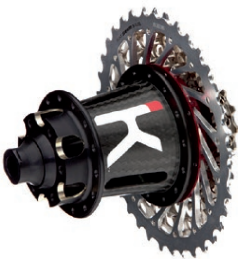
The Kappius rear hub is a groundbreaking lightweight, durable, oversized design. Its carbon-fiber housing contains a drivetrain assembly comprised of three components including an inner pawl ring, a toothed drive ring, and pawls. The components are all manufactured from an extremely durable tool steel using Direct Metal Laser Sintering (DMLS) (Source: Kappius Components).
